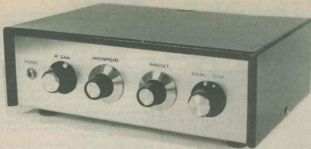
The use of a ready-made metal case makes the construction of this simple short wave superhet even simpler. Plug-in coils obviate the necessity for a wave band switch
