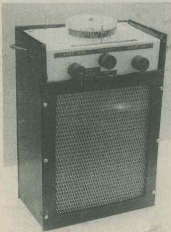
The completed "Watersport" receiver. The tuning control is at the top and is fitted with a simple home constructed tuning scale
